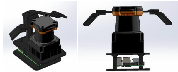
Figure 7: Dual purpose mechanism: 2D SLAM and local altitude measurement
